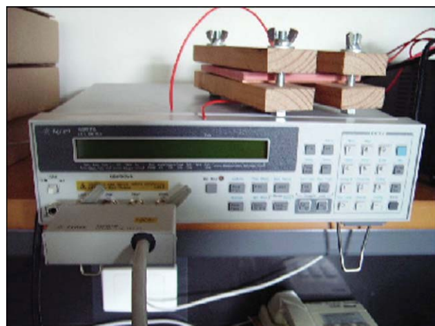
Figure 2 The Agilent 4263B LCR meter with the parallel plate capacitor and sample ready for testing. [Color figure can be viewed in the online issue, which is available at wileyonlinelibrary.com .]
